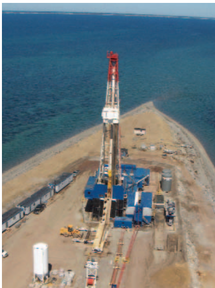
The Green Point play is enclosed by the land of the peninsula and can be entirely developed by land-based horizontal drilling. (Image courtesy of Canadian Imperial)
